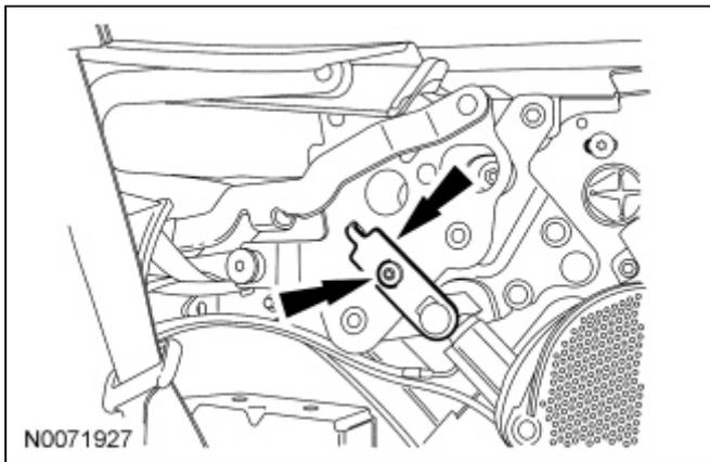
7. Remove the LH and RH clevis-to-hydraulic lift cylinder rod bolts.
